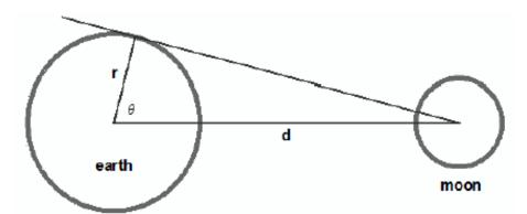
Suppose the estimate is made at a time when the equators of the earth and the moon are lined up. Then imagine a line drawn from the center of the moon tangent to the earth's surface. Measure the angle  $\theta$  – it is the latitude of the point of tangency. Then  $\cos\theta = \frac{r}{d}$ , or  $d = \frac{r}{\cos\theta}$ . Hipparchus obtained the value of 238, 000 miles, where the actual mean value is 240, 290 miles.
