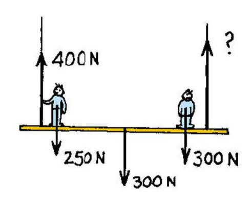
The upward forces are (400 N + RH tension). By the equilibrium rule  $\Sigma$  F = 0, this upward total must equal the downward forces are (250 N + 300 N + 300 N) = 850 N. Hence, RH tension must be 450 N.
