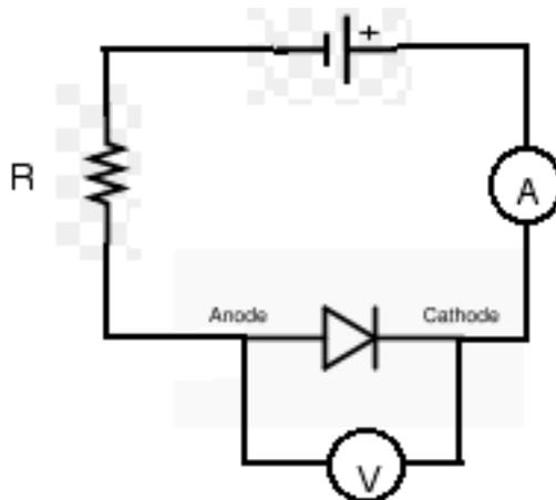
The battery would like the current to flow clockwise in the circuit and the current would do so if there were no diode in the circuit and a plain wire were in its stead. However, there is in fact a diode in the circuit and since it is in the "reverse direction" no current should flow. Check to make sure  $I_0=0$  in this case. Also, measure the voltage across the diode which should be zero also.
