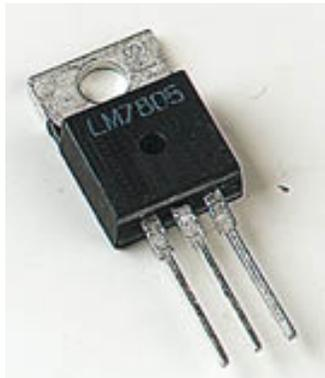
Typically voltage regulators are available as 5, 12, and 15 volts or even variable output voltages. Some regulators keep the output current fixed.
