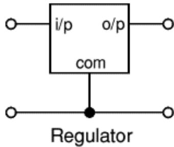
The bottom lead is common to both the input and output to the regulator. The i/p terminal is connected to the filter of the power supply and the regulated output appears at o/p. The actual regulator can appear as below
