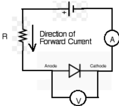
Notice the diode and battery are connected so the current flows in the forward direction. Choose a resistor  $R=5,000 \Omega$  or so the current is relatively small when the battery voltage is  $V=12$  volts. The current in this case is
