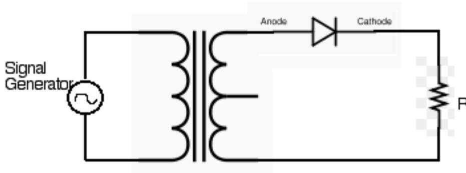
You can use your transformer in a voltage stepup mode. Again use a resistor something like  $R=5,000 \Omega$  to make the current in the milliamperes range. Connect channel #1 of your oscilloscope across the secondary of the transformer and you should see something like the diagram below:
