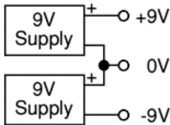
What you actually see is a power supply with three output terminals as indicated by the diagram below:
