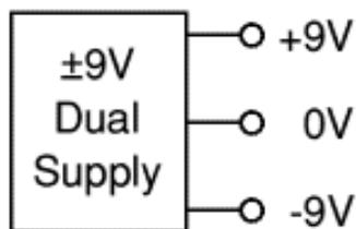
Here the three output terminals are +9 volts, 0 volts, and -9 volts. The 0 volt terminal is not necessarily grounded.
