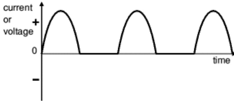
Notice that the current or voltage across the resistor is only in one direction (called positive). Only half of the original wave appears across the resistor and this kind of power supply is called a Half Wave Power Supply.
