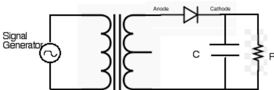
The purpose of the capacitor is to smooth the output voltage (and current) of the power supply. If you choose the proper value for the capacitor  $C$ , then the voltage (and current) across the resistor should appear as below:
