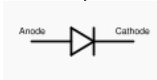
and the arrow is in the forward direction which has a low resistance. Sometimes on the physical diode, all you see is a band and this represents the bar in the above symbol.
