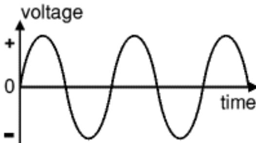
Notice the shape of the Sine wave you measure in channel #1. The frequency should be the same as the signal generator and make sure you understand the amplitude of the voltage you measure across the secondary of the transformer in terms of the turns ratio of the transformer and the amplitude of the input voltage applied to the primary.
