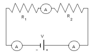
The voltage across each resistor is **different** for the case of resistors in series. For example, the voltage across resistor  $R_1$  is determined with a voltmeter as indicated below:
