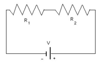
If two resistors are in **series**, then same current i flow through each resistor. Suppose for example, the voltage source V=12 volts and the resistors have values  $R_1 = 10,000 \Omega$  and  $R_2 = 20,000 \Omega$ . (You should repeat this experiment using two resistors in your parts box. Make sure the resistors are large enough so that the current is smaller than 1 milliampere otherwise you might blow a fuse in your ammeter, "fry" (burn out) a resistor, or meltdown your power supply.)
