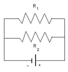
If two resistors are in **parallel**, then same **voltage** is across each resistor. The total resistance of two resistors in parallel is given by
