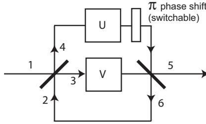
Figure 4. Testing whether two transforms commute or anticommute with an interferometric set-up. The photon is recycled so that one of the output ports (mode 6) is connected into one of the input ports (mode 2). The phase shift of  $\pi$  can be turned on during the second passage in order to reverse the output modes, so that we can test either for commutativity or anticommutativity in the ‘free’ output port.
