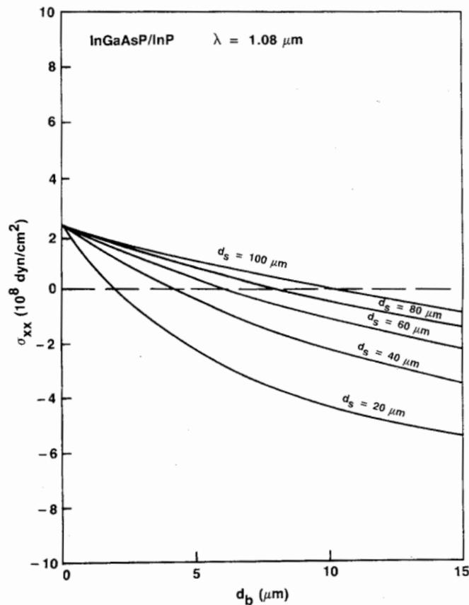
Fig. 7. Same plot as Fig. 6 for a laser at  $1.08 \mu\text{m}$  ( $y = 0.3$ ).
