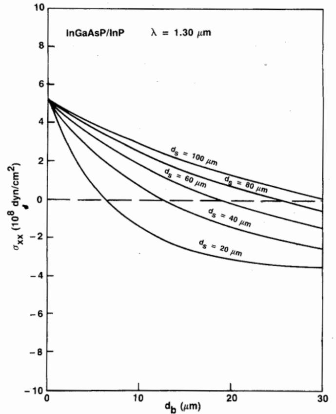
Fig. 6. Active layer stress at room temperature for a laser at  $1.3 \mu\text{m}$  ( $y = 0.6$ ) with the structure of Fig. 3(a), grown perfectly lattice-matched at  $650^\circ\text{C}$ , as a function of the buffer layer thickness for various substrate thicknesses.
