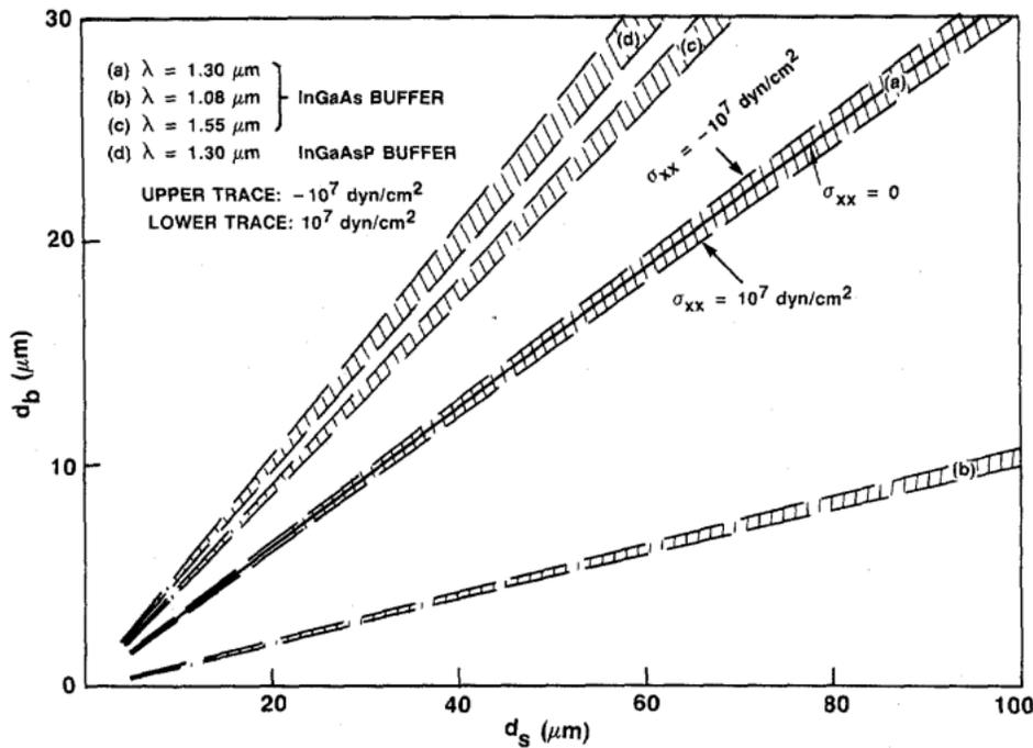
Fig. 9. Optimal relationships between the thicknesses of the buffer layer and the substrate for the stress-free condition for (a) 1.3  $\mu\text{m}$ , (b) 1.08- $\mu\text{m}$ , (c) 1.55- $\mu\text{m}$  structures with an InGaAs buffer layer, and (d) a 1.3- $\mu\text{m}$  structure with an  $\text{In}_{0.74}\text{Ga}_{0.26}\text{As}_{0.60}\text{P}_{0.40}$  buffer layer. Each pair of traces shows a stress tolerance of  $\pm 10^7$  dyne/cm<sup>2</sup>.
