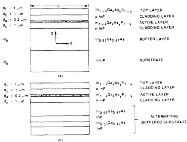
Fig. 3. (a) Improved InGaAsP/InP laser structure with an InGaAs buffer layer. (b) Buffered InGaAsP/InP laser structure with alternating InGaAs and InP layers.
