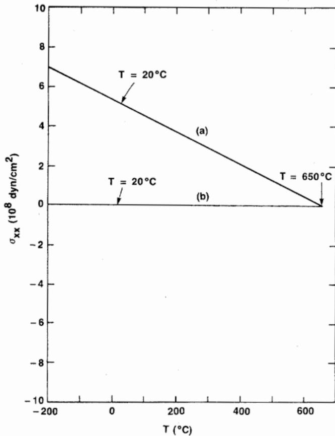
Fig. 5. Temperature dependence of the active layer stress of lasers at  $1.3 \mu\text{m}$  which have (a) a structure of Fig. 1(a) with any substrate thickness and (b) a structure of Fig. 3(a) with optimal  $d_b$  and  $d_s$  for the stress-free condition, both grown under perfect lattice-matching conditions at  $650^\circ\text{C}$ .
