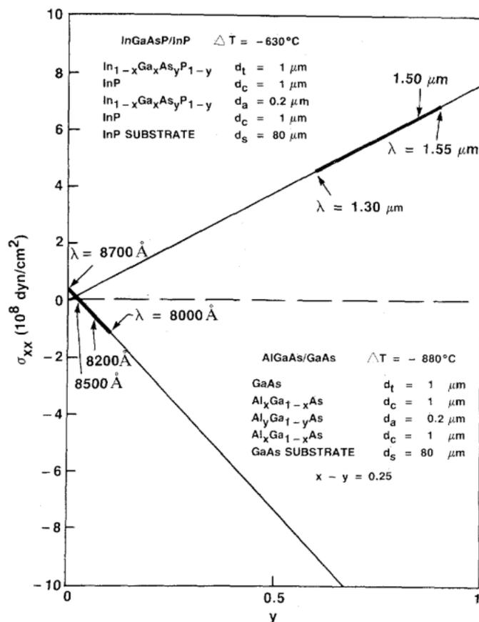
Fig. 2. Active layer stress at room temperature for the structures of Fig. 1, grown under perfect lattice-matching conditions at  $650^\circ\text{C}$  and  $900^\circ\text{C}$  for InGaAsP/InP and AlGaAs/GaAs, respectively.  $y$  refers to the As content in the cladding layers of the InGaAsP/InP structure and the Al content in the active layer of the AlGaAs structure, respectively.
