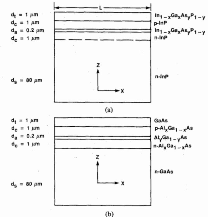
Fig. 1. Schematic structure of (a) a typical conventional InGaAsP/InP laser and (b) a typical conventional AlGaAs/GaAs laser.
