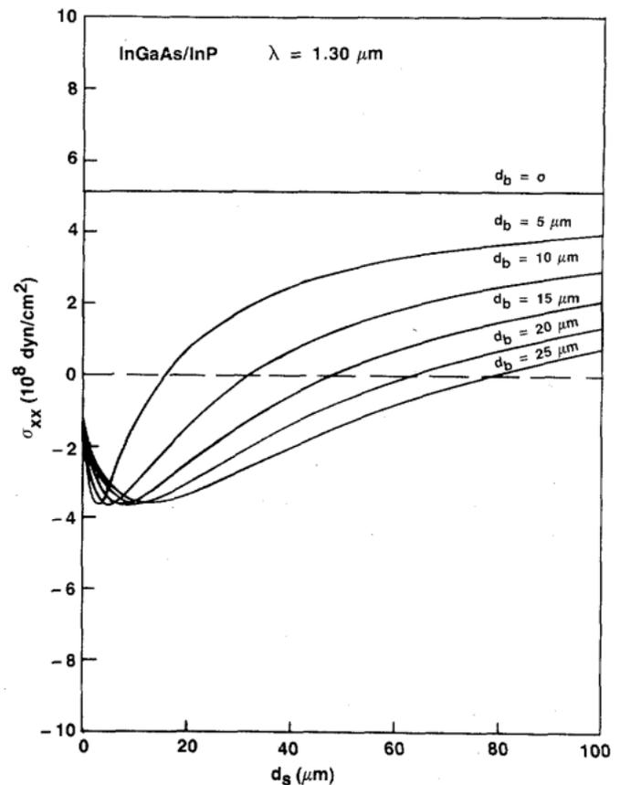
Fig. 4. Active layer stress at room temperature for a laser at  $1.3 \mu\text{m}$  ( $y = 0.6$ ) with the structure of Fig. 3, grown perfectly lattice-matched at  $650^\circ\text{C}$ , as a function of the substrate thickness for several thicknesses of the buffer layer.
