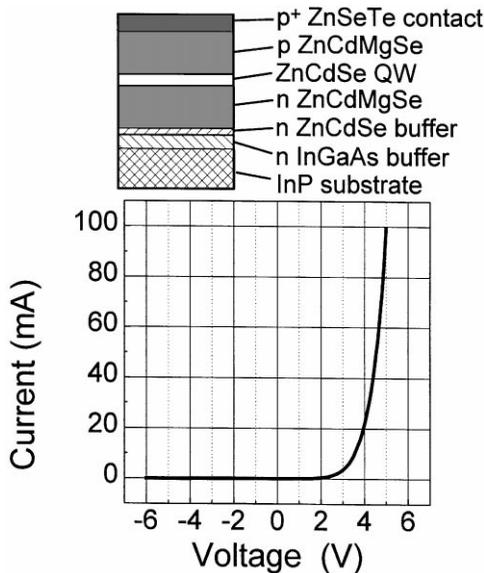
Fig. 2. Current-voltage ( $I$ - $V$ ) characteristics of a ZnCdMgSe-based LED structure. The top contact is a Au dot ( $\sim 0.3$  mm<sup>2</sup>). The top shows a schematic of the LED layer structure grown. Similar  $I$ - $V$  characteristics were obtained with samples having a 1000 Å or 200 Å thick ZnSeTe p-contact layer.
