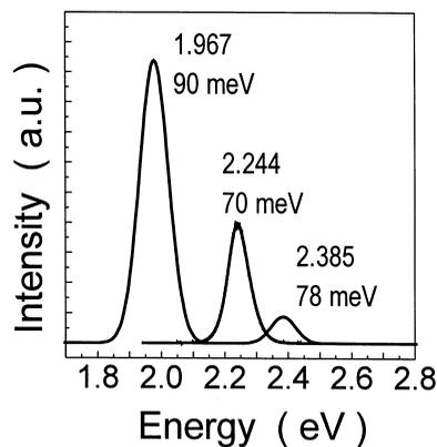
Fig. 3. Surface electroluminescence (EL) spectra for three LED structures that differ only in the QW thickness and/or composition used. Emission throughout the visible range is observed.
