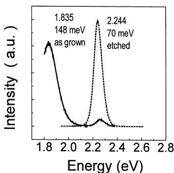
Fig. 4. Surface electroluminescence (EL) spectra for an LED structure with a thick (1000 Å) ZnSeTe p+ contact layer (solid line). The dashed line represents the EL for the same structure after etching the top ZnSeTe layer to 150 Å. The broad red emission in the as-grown structure originates from the ZnSeTe cap layer and not from the QW.
