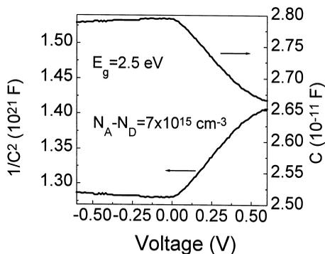
Fig. 1. Capacitance–voltage ( $C-V$ ) plot for a  $\text{ZnCdMgSe}$  quaternary layer with bandgap of 2.5 eV doped with nitrogen. The  $N_A - N_D$  level is  $7 \times 10^{15}/\text{cm}^3$ .
