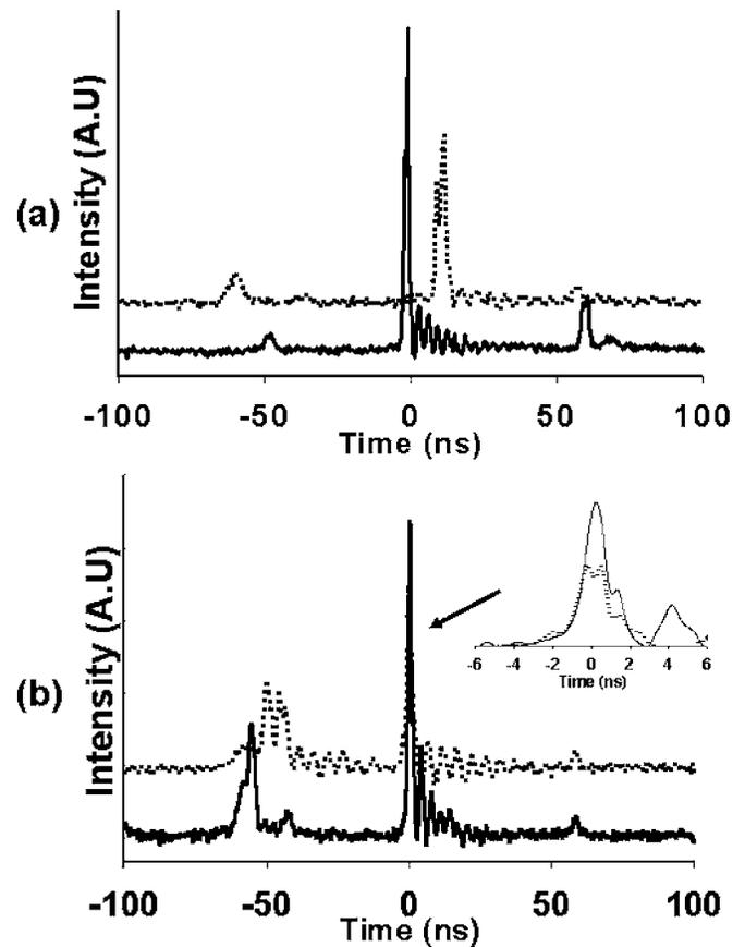
FIG. 3. Oscilloscope traces of the laser pulses from two fiber lasers when they are phase (a) unlocked and (b) locked.
