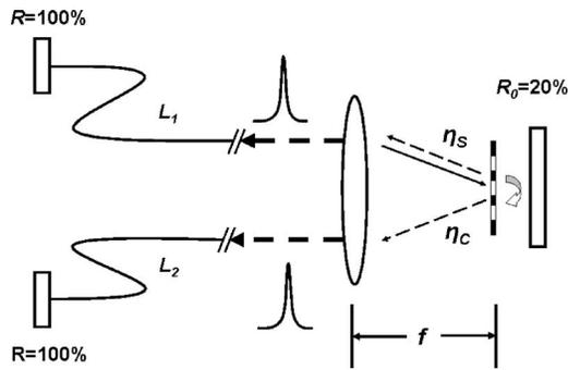
FIG. 4. Two-element laser coupled through a diffractive element in an external resonator.
