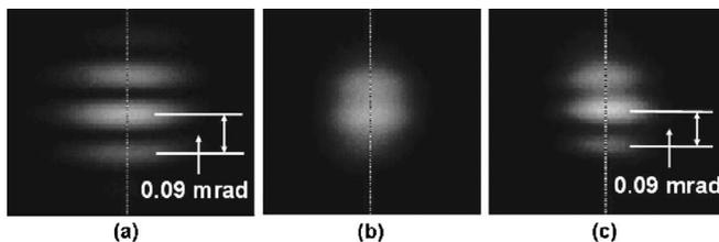
FIG. 2. Beam profiles at the output mirror of (a) phase-locked  $Q$ -switched laser pulses, (b) free-running SBS pulses, and (c) phase-locked SBS pulses.
