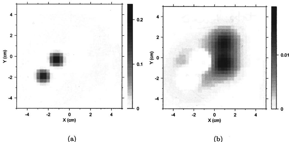
Fig. 9. Layer reconstruction at a noise level of 5%: (a) resolved objects E (left) and F (right) at  $z = 0.75 \text{ cm}$  (layer 3); (b) resolved objects G (upper) and H (lower) at  $z = 1.35 \text{ cm}$  (layer 5). The darkness of the pixel represents the resolved reduced scattering coefficient in units of inverse millimeters.
