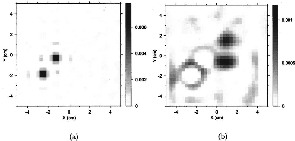
Fig. 4. Layer reconstruction at a noise level of 1%: (a) resolved objects A (left) and B (right) at  $z = 0.75$  cm (layer 3); (b) resolved objects C (upper) and D (lower) at  $z = 1.95$  cm (layer 7). The darkness of the pixel represents the resolved absorption coefficient in units of inverse millimeters.
