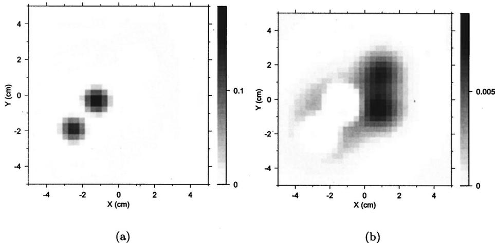
Fig. 10. Layer reconstruction at a noise level of 10%: (a) resolved objects E (left) and F (right) at  $z = 0.75 \text{ cm}$  (layer 3); (b) resolved objects G (upper) and H (lower) at  $z = 1.35 \text{ cm}$  (layer 5). The darkness of the pixel represents the resolved reduced scattering coefficient in units of inverse millimeters.
