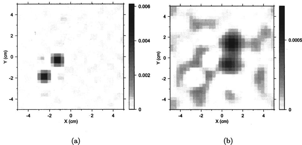
Fig. 5. Layer reconstruction at a noise level of 5%: (a) resolved objects A (left) and B (right) at  $z = 0.75$  cm (layer 3); (b) resolved objects C (upper) and D (lower) at  $z = 1.95$  cm (layer 7). The darkness of the pixel represents the resolved absorption coefficient in units of inverse millimeters.
