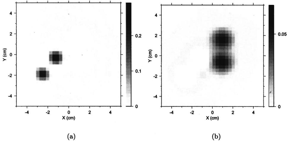
Fig. 8. Layer reconstruction at a noise level of 1%: (a) resolved objects E (left) and F (right) at  $z = 0.75$  cm (layer 3); (b) resolved objects G (upper) and H (lower) at  $z = 1.35$  cm (layer 5). The darkness of the pixel represents the resolved reduced scattering coefficient in units of inverse millimeters.
