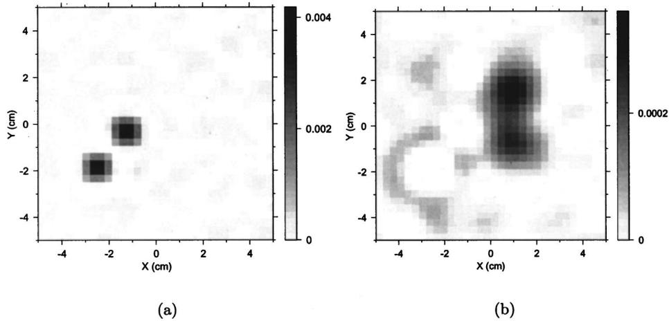
Fig. 6. Layer reconstruction at a noise level of 10%: (a) resolved objects A (left) and B (right) at  $z = 0.75$  cm (layer 3); (b) resolved objects C (upper) and D (lower) at  $z = 1.95$  cm (layer 7). The darkness of the pixel represents the resolved absorption coefficient in units of inverse millimeters.
