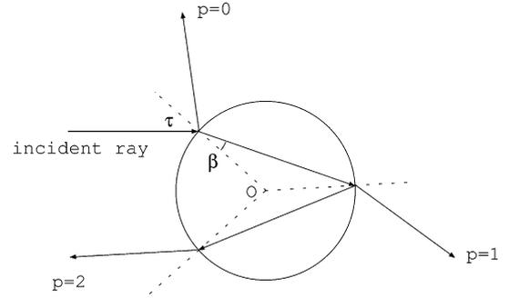
Fig. 1. Geometrical rays scattered by a sphere.
