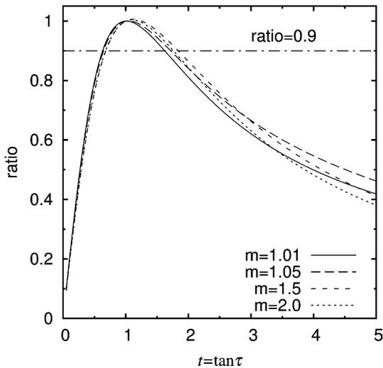
Fig. 2. The ratio  $(A_{R_1} \sin \frac{\theta}{2}) / (A_{R_1} \sin \frac{\theta}{2})_{t=1}$  versus  $t = \tan \tau$ . The curves obtained for particles of different refractive indices intersect with the 90% line at  $t \simeq 0.7$  and  $t \simeq 1.6$  where the value of the incidence angle is  $\tau = 0.2\pi$  and  $\tau = 0.3\pi$ , respectively.
