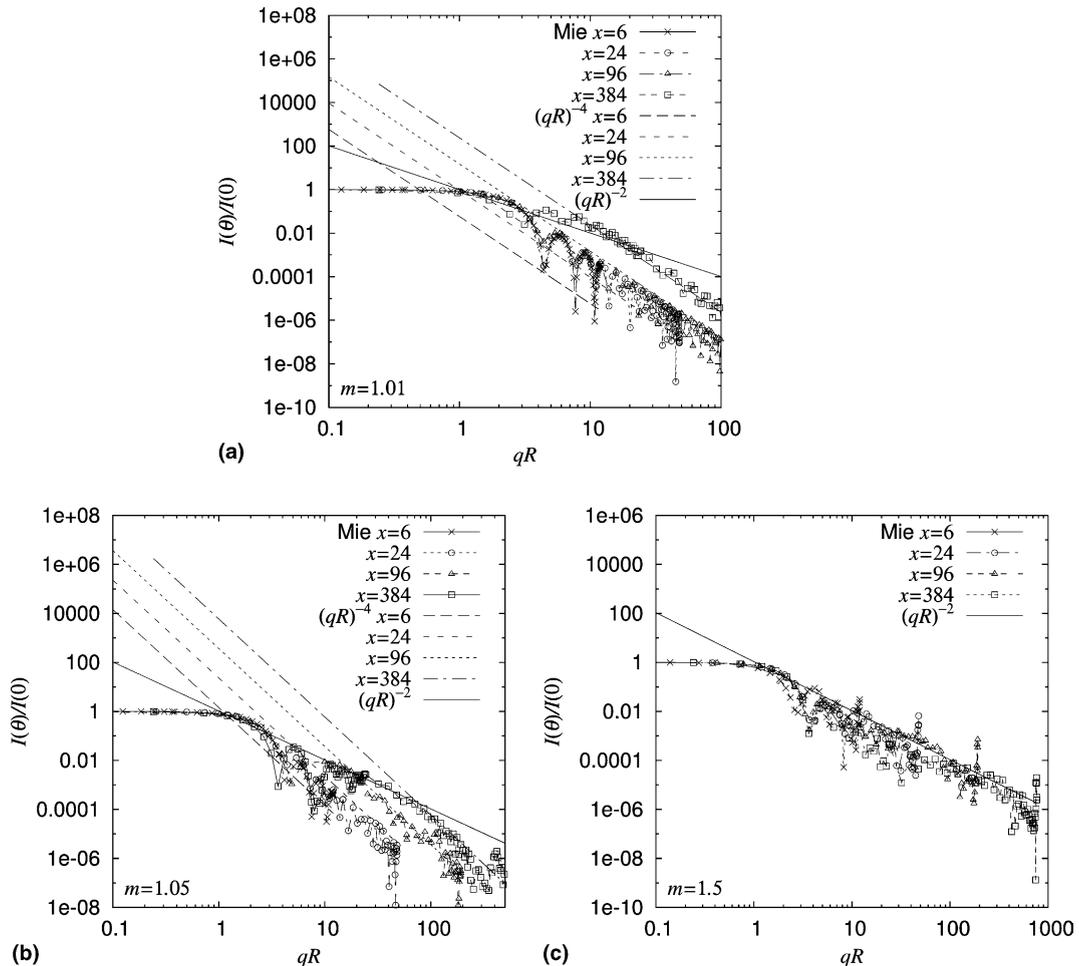
Fig. 4. The normalized Mie scattering curves plotted versus  $qR$  for spheres of refractive index: (a)  $m = 1.01$ ; (b)  $m = 1.05$ ; (c)  $m = 1.5$ . The  $(qR)^{-2}$  and  $(qR)^{-4}$  powerlaw regimes of Mie scattering given by Eq. (10) are also plotted.
