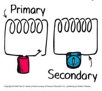
The primary coil has a battery, so when switch is closed, current flows in it, creating a sudden magnetic field that threads the secondary coil – inducing current pulse in it too. (Note no battery in secondary coil).
