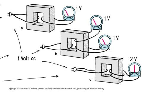
Eg. If secondary has less # turns than first, the voltage induced will be less, ie. *stepped down*.
