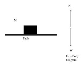
There two force acting on the mass M as indicated in the free-body diagram.
