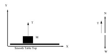
The free-body diagram is on the right and there are now three forces in the ydirection (and none in the x-direction). The total force acting on the mass M is  $F_y = N + T - W$  and Newton's 2nd Law appears
