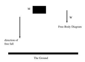
A "Free-Body Diagram" is shown to the right of the falling mass. The "Free-Body Diagram" does not show the falling body (hence the diagram is free of the body) and only the force(s) acting on appear. In this case there is only one force W. Newton's 2nd law  $\vec{F} = m \vec{a}$  for this problem is W = M g
