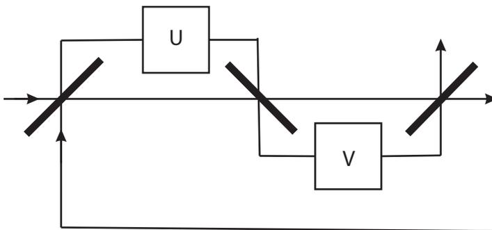
Figure 3. Interferometric comparison involving a single photon and two interferometers connected in series, with recycling of the photon.
