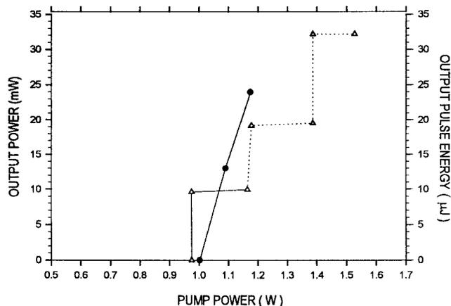
Fig. 2. CW output power (circles) and quasi-CW pulse energy (triangles) versus pump-power characteristics of a monolithic Q-switched Cr-Nd:YAG laser operating at 946 nm. The single-frequency (solid lines) and two-frequency (dotted lines) regions are indicated. The triangles are experimental points.
