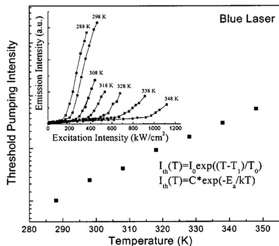
FIG. 6. Temperature dependence of the lasing threshold for blue laser structure. Lasing is observed up to 348 K and  $T_0$  is estimated to be 35 K.
