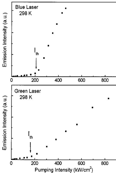
FIG. 4. Output intensity vs pumping intensity at room temperature. The threshold excitation intensity is estimated to be  $\sim 220$  kW/cm<sup>2</sup> for the blue laser and  $\sim 160$  kW/cm<sup>2</sup> for the green laser.
