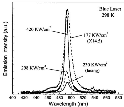
FIG. 5. Spectra of blue laser emission at different excitation intensities operated at room temperature. (The spectrum at pumping intensity of 177 kW/cm<sup>2</sup> is amplified by 14.5 times in order to see clearly the emission from barrier.)
