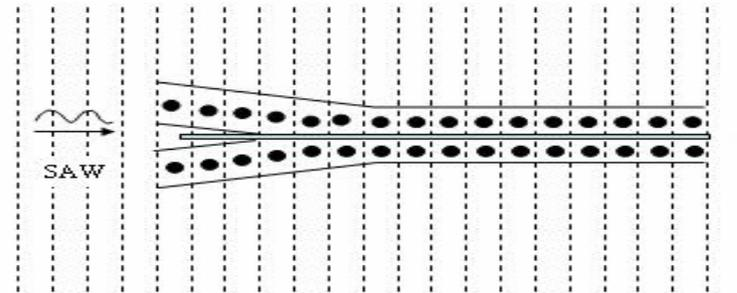
Two electrons, moving along narrow adjacent channels, are captured by a SAW and form a pair of coupled quantum dots. The full circles denote electrons. .
