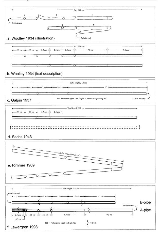
Fig. 1 Various reconstructions of the two main silver pipes.
