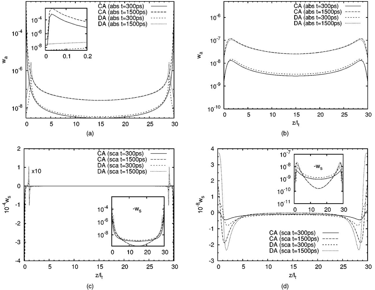
FIG. 7. Weight function for a slab where the inhomogeneity is (a) absorption and (c) scattering at  $(0,0,z)$ , in the propagation direction of the source, (b) absorption and (d) scattering at  $(0,l_t,z)$ , off by one transport mean free path. Weight functions calculated from the cumulant (CA) and diffusion (DA) approximations are plotted for time delays of  $t=300$  ps and  $t=1500$  ps. The insets replot the weight functions in a logarithm scale.
