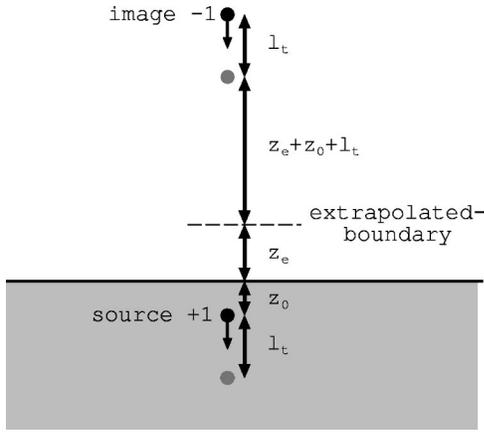
FIG. 1. The incident source at position  $(x_0, y_0, z_0 \geq 0)$  and its image source at  $(x_0, y_0, -z_0 - 2z_e - 2l_t)$  propagating along the positive  $z$  axis in a semi-infinite medium ( $z \geq 0$ ) with its interface at  $z=0$ . The source and its image move from their original positions (dark spots) to their final stops (shadow spots) at later times.
